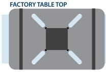
The through slot table top is the most common factory table top and allows the Fulton Deluxe Table top to be mounted using the included post knob and bolt hardware.
