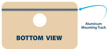
The Aluminum Mounting Track that is secured to the bottom of the drill press table makes mounting the Deluxe Drill Press Table quick and easy.
